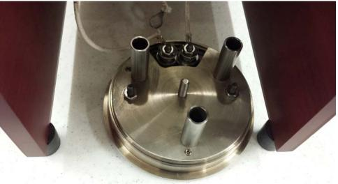
22. Place the three spacers on the heater head plate directly over their respective socket.
