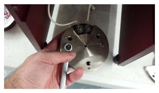
15. Using a 3/8 wrench remove the two hex nuts holding the heating element to the heater head plate.
