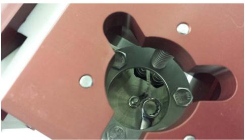
8. Using a 7/16 wrench remove the hex nut on the top of the heater head. There is a ground wire going to the center of the heater head plate underneath that hex nut. You may also try this with a ratchet wrench and an extension.
