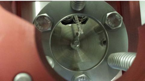
25. Replace the ground wire to the center bolt.
