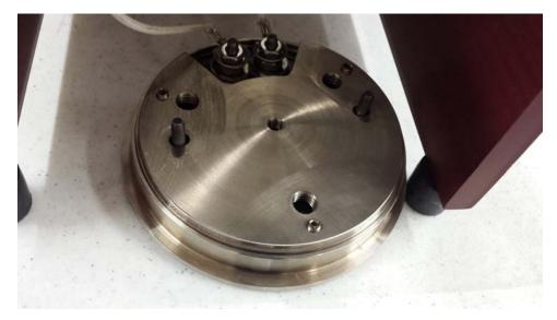
18. Now plate the heat seal head onto the heater head plate, with the heating element between the two. Make sure the heater head plate is seated level into the heat seal head.
