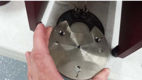
16. Remove the plate and locate the three set screws.
