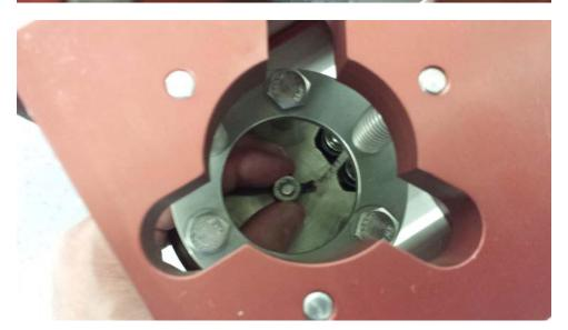
26. Replace the hex head nut to hold the ground wire down to the heater head plate.
