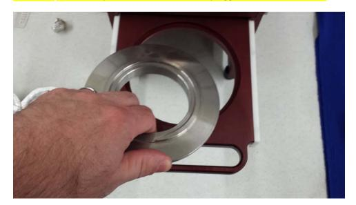
1. Ensure the unit is cool, powered off and unplugged. Then remove the nest insert.
