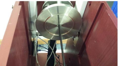
11. Use a 5/32 hex wrench or hex key to remove the bolt in the center of the sealing head.
