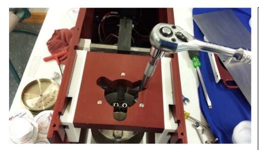
13. Using a 9/16 ratchet wrench remove the 3 bolts holding the heater head plate.
