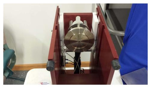
10. Now turn the unit on its back. This gives you access to the bottom side of the sealing head.
