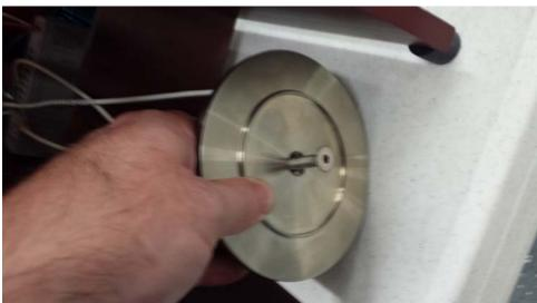
19. Now put the flat head bolt through the bottom. This will help ensure everything is aligned properly. Tighten down properly. This will sandwich the heating element between to heat seal head and the heater head plate.
