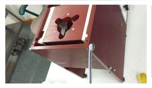
6. With a 5/16 wrench remove the four bolts that hold the front cover on.
