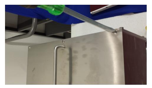
30. Replace the 6 screws that hold the top cover down.
