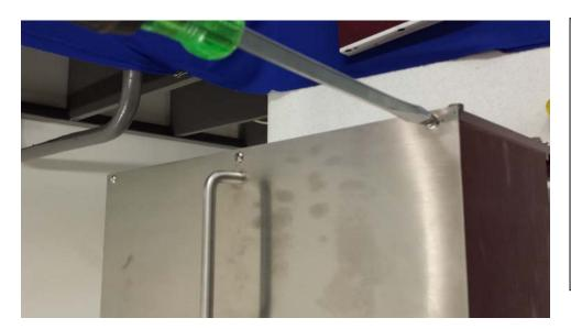
4. Remove the 6 screws that hold the top cover down.
