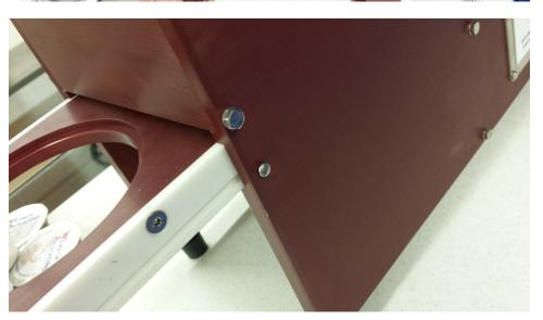
32. Turn the two screws on the side back in so that the nest tray will not slide all the way out.
