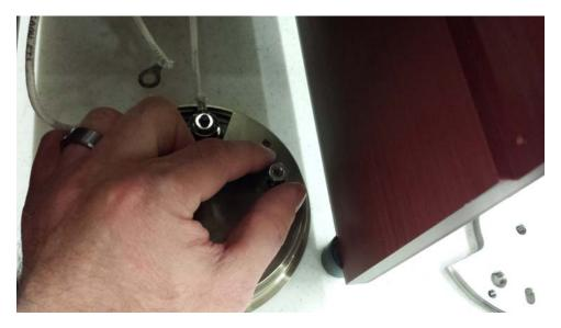
21. Now replace the two hex head nuts to the two prongs of the heating element to lock it in place.
