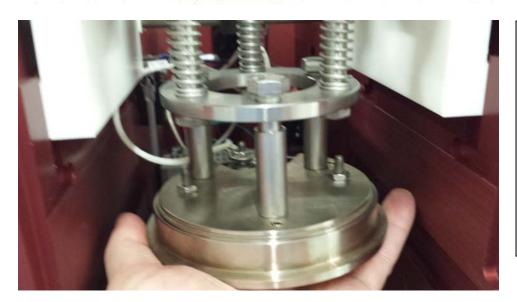
23. Carefully raise the heater head assembly so that the spacers cover their three respective bolts.
