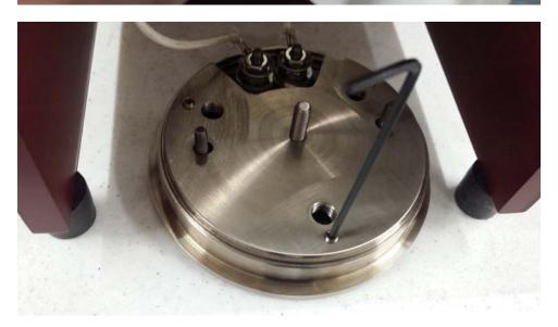
20. Now you may turn the set screws through until they stop. This ensures that the heating element is pushed against the heat seal head for maximum heat transfer.
