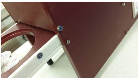
2. Locate the two screws that hold the nest tray from sliding out and with a flat head screw driver turn them back far enough to allow the tray to slide completely out.
