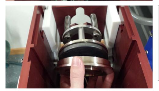
12. Remove the sealing head from the heater head plate.
