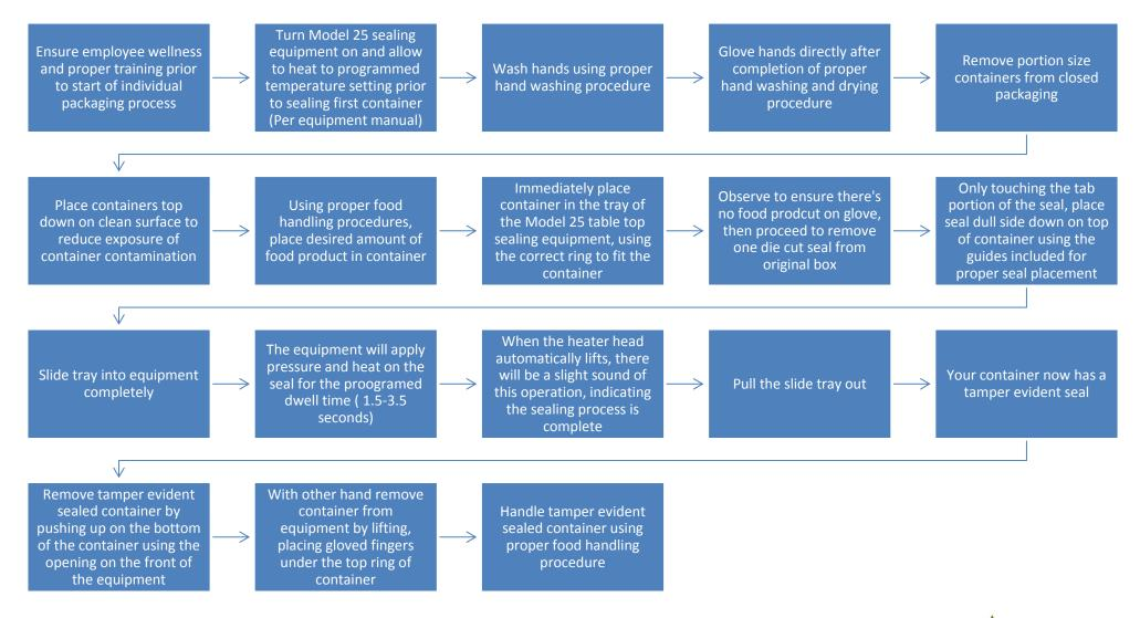
This procedure can be incorporated into any comprehensive HACCP plan. The Wilpack Packaging Tamper Evident Sealing Equipment is a useful tool used to control exposure of contamination or adulteration of food products for human consumption.
